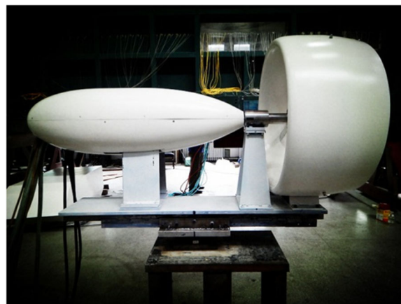
Fig. 4 Model of ducted fan experiment
