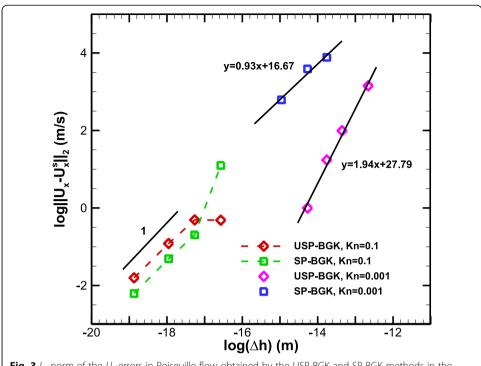
**Fig. 3**  $L_2$ -norm of the  $U_x$ -errors in Poiseuille flow obtained by the USP-BGK and SP-BGK methods in the continuum (Kn = 0.001) and rarefied (Kn = 0.1) flow regimes
