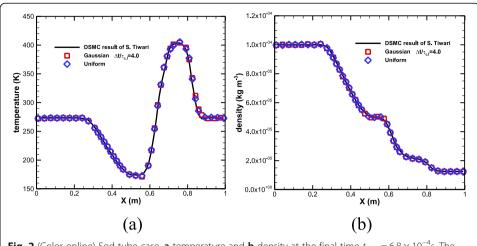
**Fig. 2** (Color online) Sod tube case. **a** temperature and **b** density at the final time  $t_{final} = 6.8 \times 10^{-4}$ s. The solid lines are results of DSMC obtained by S. Tiwari [27] and the symbols refer to the efficient USP-BGK results
