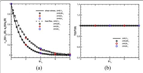
**Fig. 1 a** relaxation of shear stress and heat flux; **b** temperature evolution in the homogeneous flow with four different time step size  $\Delta t \in \{0.1\tau_C, 0.25\tau_C, 2.0\tau_C, 4.0\tau_C\}$ .
