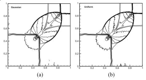
**Fig. 5** Density distribution of the 2D Riemann problem using the efficient USP-BGK method with **a** Gaussian and **b** uniform kernel functions
