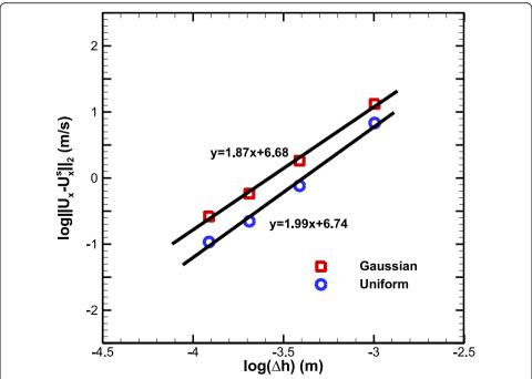
**Fig. 4**  $L_2$ -norm of the  $U_x$ -errors for the efficient USP-BGK method in the Taylor-Green vortex flow depended on the cell size, and  $\Delta h \in \{1/50, 1/40, 1/30, 1/20\}$  (m). The uniform and Gaussian kernel functions are employed
