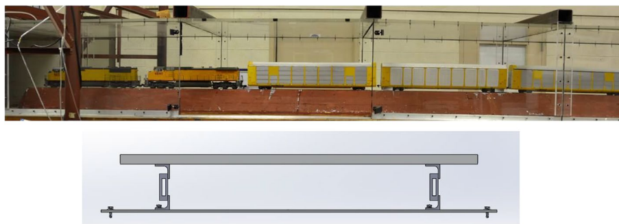
Fig. 5 Image of a train set in the wind tunnel (top) and a schematic of a track section, with accompanying load cells, on which one car from the train set was mounted (bottom)
