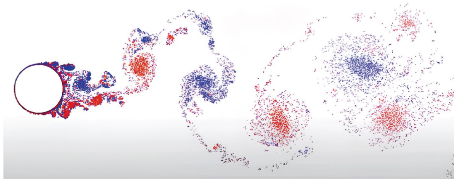
Fig. 1 Viscous fluid past a bidimensional circular cylinder through the full vortex cloud method (VCM) with random walk method for viscous diffusion calculation [1]
