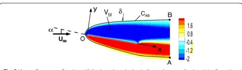
Fig. 8 Viscous flow over a flat-plate airfoil, where the color bar indicates the normalized vorticity. From Liu et al. [28]
