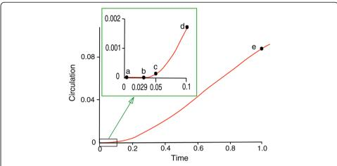
**Fig. 13** Growth of the airfoil circulation in the accelerated starting flow over a NACA-0012 airfoil, where the typical moments corresponding to the flow patterns in the circulation formation in Fig. 12 are marked. Adapted from Zhu et al. [51]
