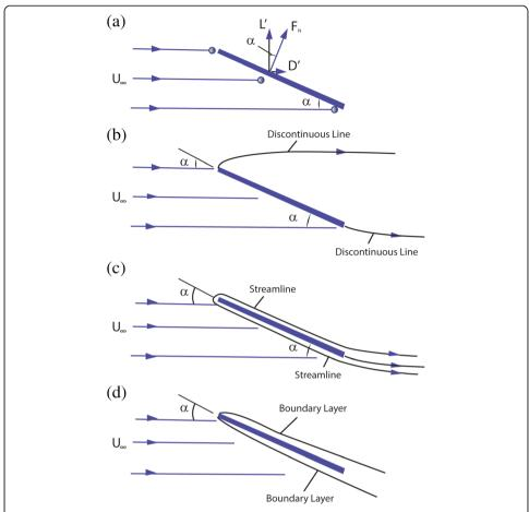
**Fig. 2** Flow patterns over a flat-plate airfoil: (a) Newton's version, (b) Rayleigh's version, and (c) thin-airfoil model, and (d) viscous-flow model
