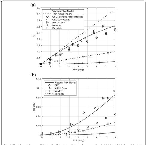
**Fig. 3** The lift and drag coefficients of a flat-plate airfoil as a function of AoA: (a) lift, and (b) drag. Adapted from Liu et al. [20].
