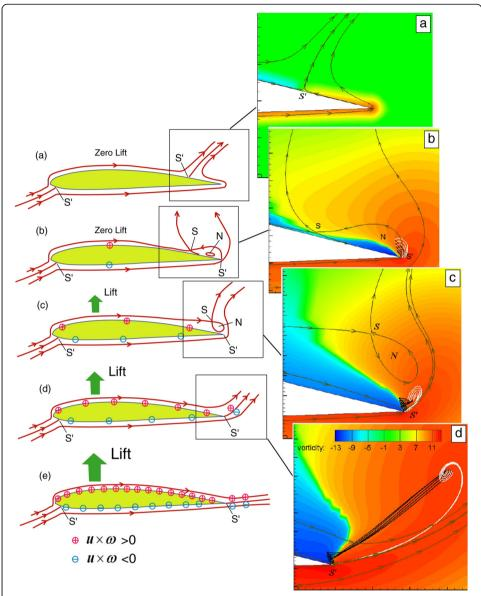
**Fig. 12** Illustration of the generic process of lift generation after the incoming uniform flow starts suddenly over an airfoil: (**a**)  $t/T_{ref} = 0.002$ , (**b**)  $t/T_{ref} = 0.029$ , (**c**)  $t/T_{ref} = 0.05$ , and (**d**)  $t/T_{ref} = 0.1$ , and (**e**)  $t/T_{ref} = 1.0$ . Streamlines, pathlines and streaklines are shown in gray lines with arrows, black lines and white lines, respectively. Adapted from Zhu et al. [51]
