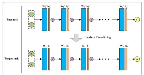
**Fig. 1** Overview of the transfer learning approach. Instead of initializing the entire network randomly, the usual transfer approach is to train a base network on a large dataset and then copy (transfer) its first *n* layers to the first *n* layers of a target network. The remaining layers are randomly initialized and trained toward the target task
