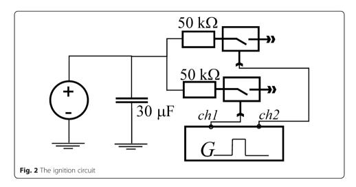
source of controlled disturbances starts charging. When the breakdown voltage is reached, a glow discharge is ignited, during burning of which the voltage drop across the electrodes remains constant. After  $10\,\mu s$ , the switch receives a zero signal and it closes, and the discharge is interrupted.
