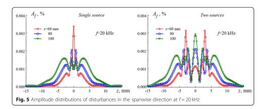
noticeable increase in disturbances at z = 0 mm, since the summation of synchronous waves is taking place in this region.
