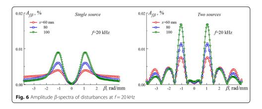
disturbances has doubled, the wave characteristics remain the same compared to the development of disturbances from a single source. In this case, for the most unstable disturbances at  $\beta = \pm 1.08 \, \text{rad/mm}$ , the angle of inclination of the wave to the incident flow was  $\pm 71^{\circ}$ , which is in accordance with previously performed experiments under controlled conditions in the supersonic boundary layer on a flat plate [16].
