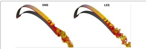
**Fig. 10** Instantaneous Q-criterion contours colored by the axial velocity. The **DNS** solution consists of 9.5M DOF using a p3 discretization on the fine mesh whereas the **LES** consists of 0.5M DOF using a p2 discretization on the coarse mesh
