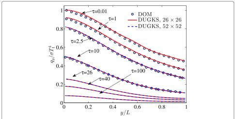
Fig. 8 Effect of optical thickness on the centerline nondimensional net radiative heat flux in the y-direction (Medium: F2,  $\rho = 0$ ,  $\omega = 1.0$ )
