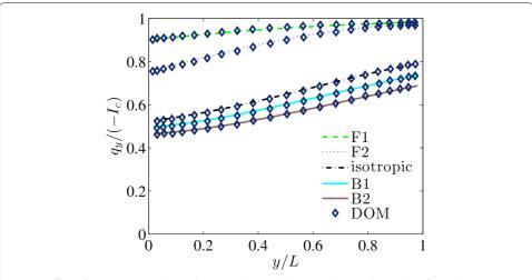
**Fig. 11** Effect of anisotropic media on the centerline nondimensional net radiative heat flux in the y-direction ( $\rho=0,\omega=1.0,\tau=1.0$ )
