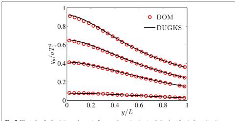
**Fig. 7** Effect of wall reflectivity on the centerline nondimensional net radiative heat flux in the *y*-direction (Medium: F2,  $\omega = 1.0$ ,  $\tau = 1.0$ )
