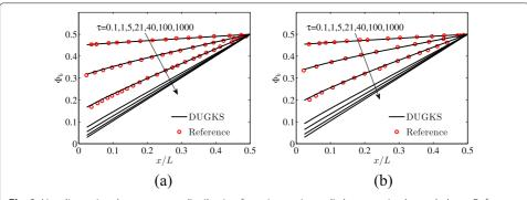
**Fig. 2** Nondimensional temperature distribution for anisotropic media between isothermal plates. Reference data are taken from [43] (a) medium A, (b) medium B
