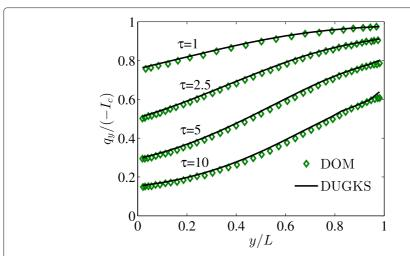
**Fig. 12** Effect of optical thickness on the centerline nondimensional net radiative heat flux in the y-direction (Medium: F2,  $\rho=0$ ,  $\omega=1.0$ )
