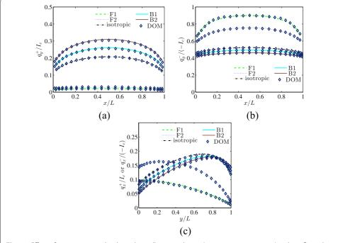
**Fig. 10** Effect of anisotropic media along the walls energy losses ( $\rho=0,\omega=1.0,\tau=1.0$ ). **a** the reflected flux loss on top wall, **b** the transmitted flux loss on bottom wall, **c** the flux loss on side walls
