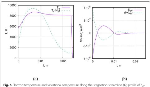
**Fig. 5** Electron temperature and vibrational temperature along the stagnation streamline (**a**); profile of  $S_{eV}$  and heat flux divergence (**b**)
