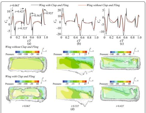
**Fig. 7** Aerodynamics, pressure distribution and flow field of the flapping wing with or without clap-and-fling effect in typical time. **a-c** lift, drag, aerodynamic power coefficient changes during a stroke cycle, **d** pressure distribution of typical time
