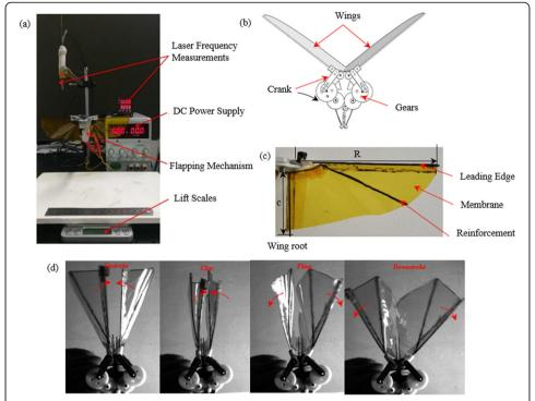
**Fig. 2** Experimental apparatus and model (**a**) the fast lift measurement platform, (**b**) experimental test model, (**c**) Wing structure, (**d**) the flapping wings with clap-and-fling motion
