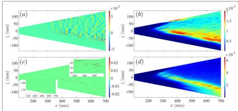
**Fig. 7** The instantaneous **a**, **c** and r.m.s. **b**, **d** of low- and high-frequency  $p_w$ . **a**, **b** for low-frequency  $p_w$  with frequency 10-50 kHz and **c**, **d** for high-frequency  $p_w$  with 300-600 kHz. Details of high-frequency  $p_w$  are given in two regions by the subfigures
