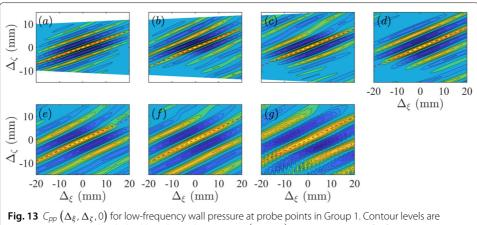
[-1:0.1:-0.2 0.2:0.1:1]. The dashed lines have slopes  $\arctan\left(\Delta_{\zeta}/\Delta_{\xi}\right)=20^{\circ}$  in **a**, 22.5° in **b**, **d**, 21.5° in **c**, 24.5° in e and 26° in f, g
