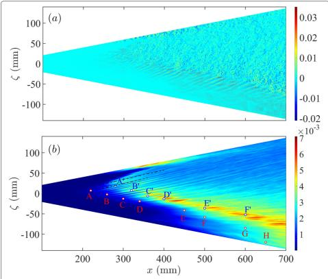
**Fig. 5** The instantaneous **a** and r.m.s. **b** of the fluctuating wall pressure. The dashed lines in **b** represent the trajectories of stationary crossflow vortices shown in Fig. 4. The markers are probe points with those upstream and downstream of the transition front labeled as Group 1 and Group 2, respectively
