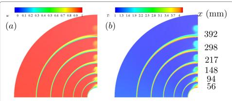
**Fig. 2** Axial slice of nondimensional u and T on the leeward side of undisturbed basic state computed by second order finite volume method
