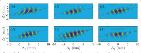
**Fig. 15**  $C_{pp}\left(\Delta_{\xi},\Delta_{\zeta},0\right)$  for high-frequency wall pressure at probe points in Group 2. Contour levels are the same as in Fig. 13. The dashed lines have slopes arctan  $\left(\Delta_{\zeta}/\Delta_{\xi}\right)=10^{\circ}$  in **a**, **b**, 12° in **c**, 15° in **d**, **e** and 8° in **f**
