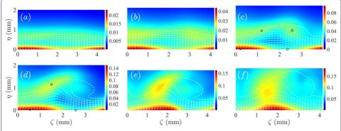
**Fig. 10** The evolution of  $p_{rms}$  in the wall-normal plane along the vortex path V2. The dashed lines represent the temporal mean axial velocity. The markers in **c**, **d** are probe points. Axial locations are from x = 220 mm to 320 mm by an increment of 20 mm
