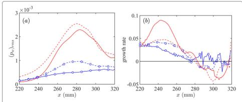
**Fig. 9** Axial evolution of  $(p_w)_{\rm rms}$  (**a**) and its growth rate (**b**) along the stationary crossflow vortex trajectories V1 (solid) and V2 (dashed). Lines with and without symbols are respectively for the low- and high-frequency wall pressure
