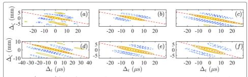
**Fig. 17**  $C_{pp}$   $\left(0, \Delta_{\zeta}, \Delta_{t}\right)$  for low-frequency wall pressure at probe points in Group 2. Contour levels are the same as in Fig. 16. The slopes of the dashed lines are  $-0.175q_{\infty}$  in **a-c**,  $-0.225q_{\infty}$  in **d**,  $-0.2q_{\infty}$  in **e** and  $-0.25q_{\infty}$  in **f**
