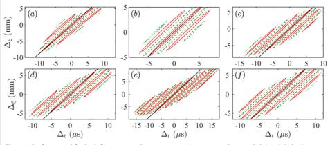
**Fig. 18**  $C_{pp}$   $(\Delta_{\xi}, 0, \Delta_{t})$  for high-frequency wall pressure at probe points in Group 2. Solid and dashed contours for 0.5 and -0.5 respectively. Solid lines represent  $\Delta_{\xi}/\Delta_{t}=0.85q_{\infty}$
