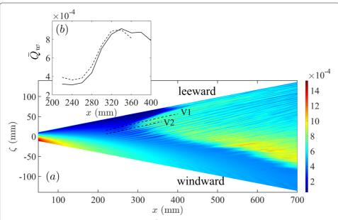
**Fig. 4 a** The temporal mean of the wall heat flux  $\bar{Q}_w$ . Dashed lines represent two trajectories of stationary crossflow vortices V1 and V2 determined by the local maximum of  $\bar{Q}_w$ .  $\bar{Q}_w$  along the two trajectories are given in **b** with solid and dashed lines respectively for V1 and V2
