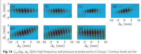
**Fig. 14**  $C_{pp}$  ( $\Delta_{\xi}$ ,  $\Delta_{\zeta}$ , 0) for high-frequency wall pressure at probe points in Group 1. Contour levels are the same as in Fig. 13. The dashed lines have slopes  $\arctan\left(\Delta_{\zeta}/\Delta_{\xi}\right)=1^{\circ}$  in **a**, 3° in **b**, 8° in **c**, 10° in **d**, 15° in **e**, 15° in **f** and 3° in **g**
