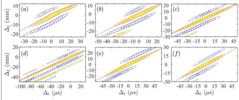
**Fig. 16**  $C_{pp}$   $(\Delta_{\xi}, 0, \Delta_{t})$  for low-frequency wall pressure at probe points in Group 2. Contour levels are [0.5:0.1:1] for solid and [-1:0.1:-0.5] for dashed. The slopes of the dashed lines are  $0.45q_{\infty}$  in **a**,  $0.5q_{\infty}$  in **b**,  $0.425q_{\infty}$  in **c**,  $0.43q_{\infty}$  in **d**,  $0.46q_{\infty}$  in **e** and  $0.45q_{\infty}$  in **f**
