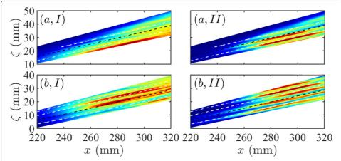
**Fig. 8** The distribution of the r.m.s. (shaded contour) of the low- (10-50 kHz, I) and high-frequency (300-600 kHz, II) wall pressure and the wall heat flux (dashed lines) in the neighbourhood of stationary crossflow vortex trajectories V1 **a** and V2 **b**. Trajectories V1 and V2 are colored in black
