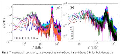
**Fig. 6** The temporal spectra of  $p_W$  at probe points in the Group 1 **a** and Group 2 **b**. Symbols denote the estimation  $f = \bar{q}_e/2\delta$
