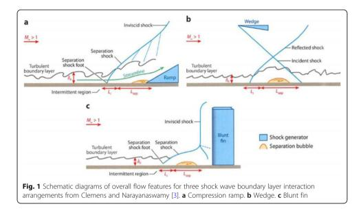
compression ramp, (b) wedge, and (c) blunt fin. Each of these results in different shock wave development and angles, as a consequence of different velocity and streamline variations relative to the imposed geometric boundaries.
