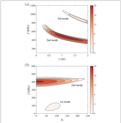
**Fig. 3** Growth rate contours  $(-\alpha_i, 1/m)$  (a) for axisymmetric waves and (b) with the azimuthal wavenumber at s = 1.6 m
