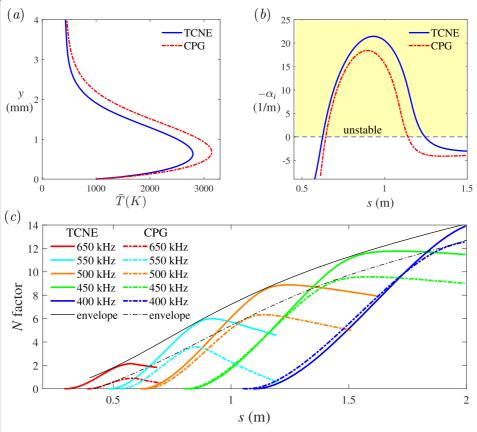
**Fig. 11** Comparisons of (a) the laminar flow profile at  $s = 0.4 \, \text{m}$ , (b) the growth rate curves with f of  $500 \, \text{kHz}$  and (c) the N factor curves between the TCNE and CPG cases
