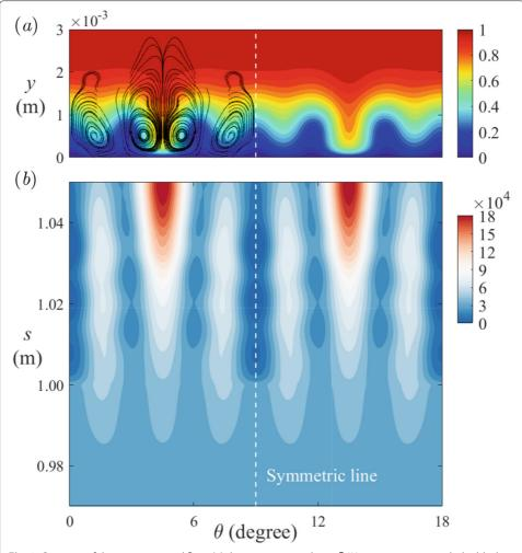
**Fig. 8** Contours of the time-averaged flow: (a) the streamwise velocity  $\bar{u}/U_{\infty}$  at  $s=1.05\,\mathrm{m}$  with the black lines the disturbance streamlines in the  $y-\theta$  plane and (b) the wall-normal gradient  $\partial \bar{T}/(T_{\infty}\partial y)$  at the wall
