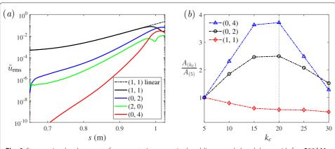
**Fig. 6** Streamwise development of representative waves in the oblique-mode breakdown with  $f = 500 \, \text{kHz}$ : (a) wave amplitudes with  $k_C = 10$  and (b) amplitude ratios at  $s = 1.02 \, \text{m}$  with  $k_C$  variation
