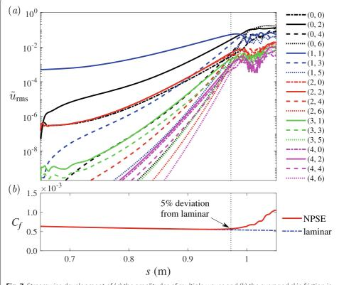
**Fig. 7** Streamwise development of (a) the amplitudes of multiple waves and (b) the averaged skin friction in the oblique-mode breakdown with  $f = 500 \, \text{kHz}$  and  $k_C = 20$
