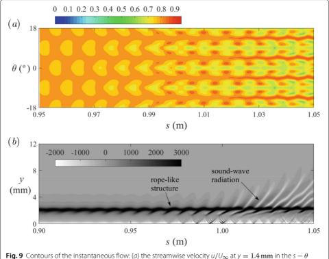
**Fig. 9** Contours of the instantaneous flow: (a) the streamwise velocity  $u/U_{\infty}$  at y=1.4 mm in the  $s-\theta$  plane and (b) the wall-normal gradient of the density  $\partial \rho/(\rho_{\infty}\partial y)$  in the s-y plane
