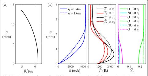
**Fig. 2** Laminar boundary-layer profiles of (a) the pressure at  $s=0.4\,\mathrm{m}$ , (b) the streamwise velocity, temperature and mass fraction at s of  $0.4\,\mathrm{m}$  and  $1.6\,\mathrm{m}$
