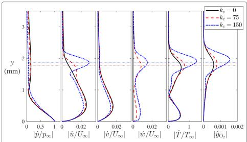
**Fig. 4** Eigenvectors of the second-mode disturbance with different azimuthal wavenumbers at s of 1 m. The disturbance frequency is 500 kHz. The subfigures are the disturbance curves of (a) pressure, (b-d) velocities, (e) temperature and (f) mass fraction of  $O_2$
