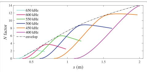
Fig. 5 N factor curves of axisymmetric second-mode waves for the disturbances with different frequencies
